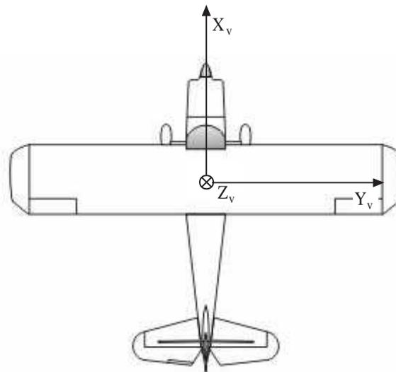
**Figure A-1:** Vehicle reference frame.
