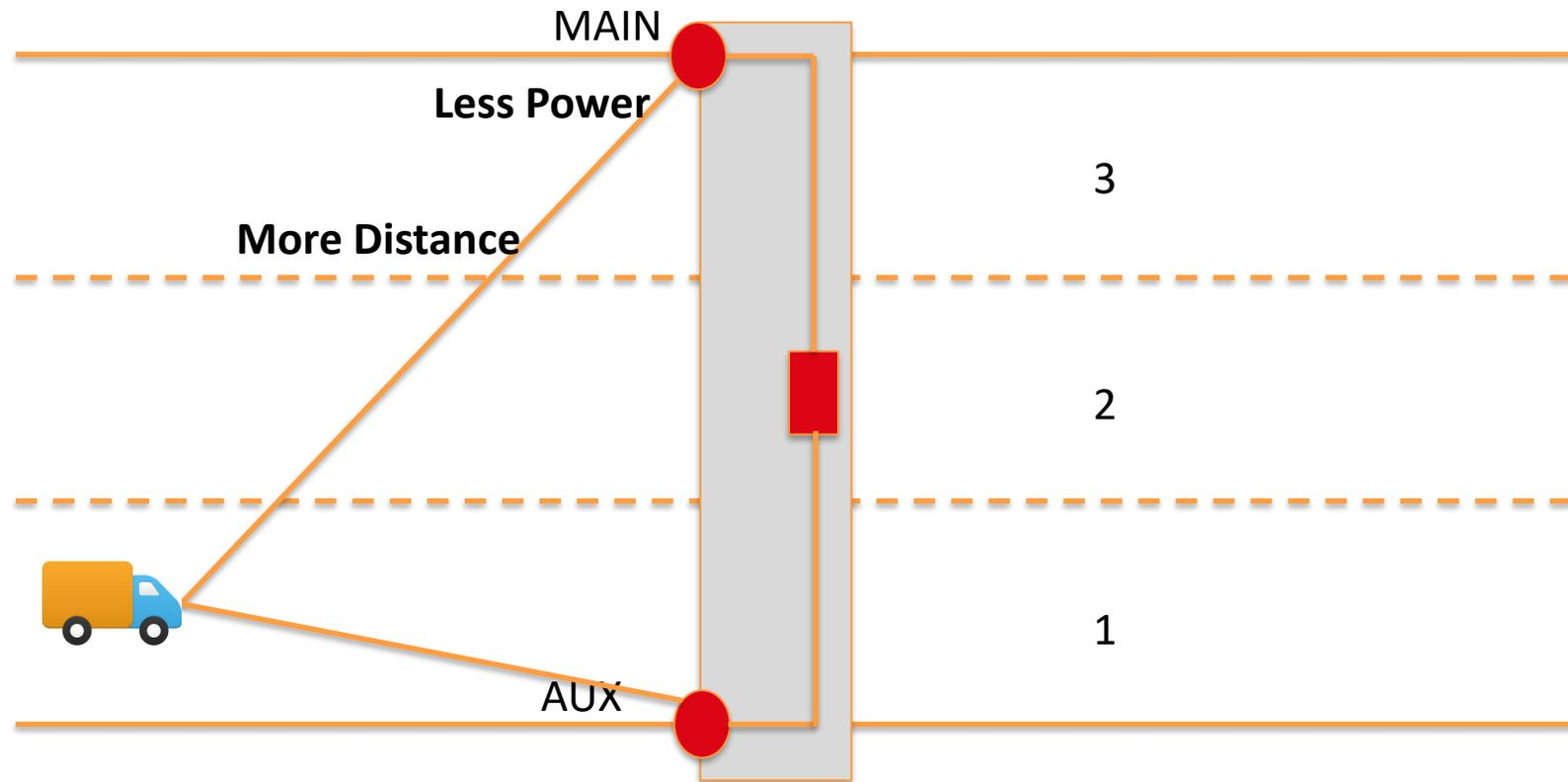
Main-Aux dtoa obtained from cross correlating the main and aux A/D samples
